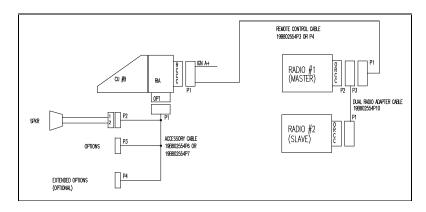
Figure 37 - Orion Dual Radio Remote Mount Installation Configuration
